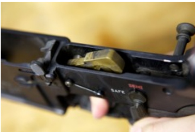
FIGURE 19 - DISCONNECTOR CATCHING THE HAMMER
