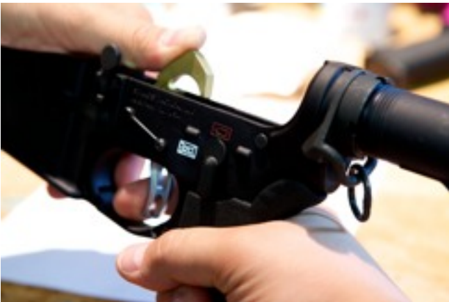
FIGURE 16 - THUMB PREVENTS DRY FIRE
