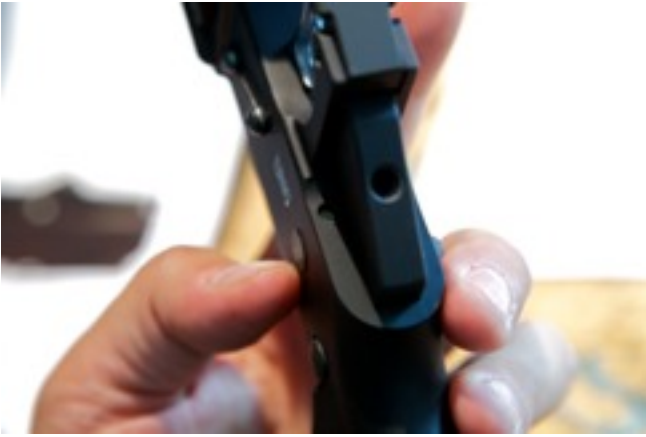
FIGURE 13 - SAFETY SELECTOR DETENT INSTALLED
