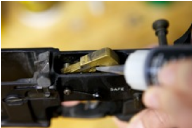
FIGURE 21 - LUBING THE HAMMER-DISCONNECTOR SURFACE
