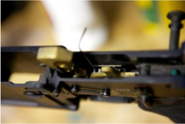
FIGURE 18 - ADJUSTMENT OF THE FRONT SET SCREW
