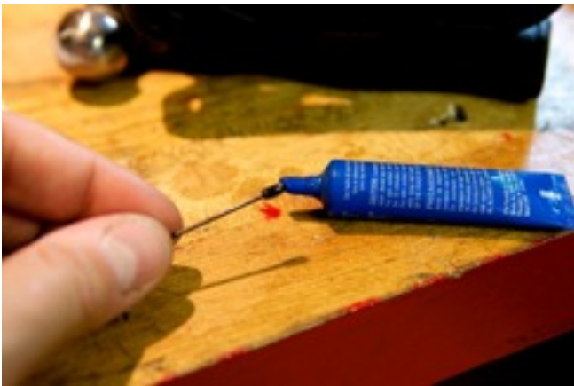
FIGURE 6 - LOCTITE SET SCREWS
