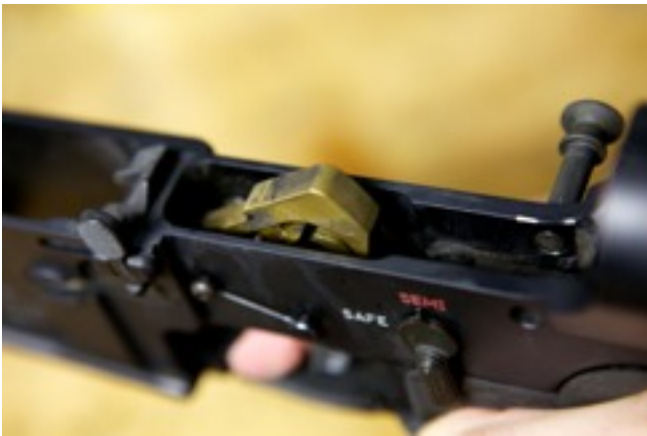
FIGURE 20 - HAMMER BACK TO READY POSITION
