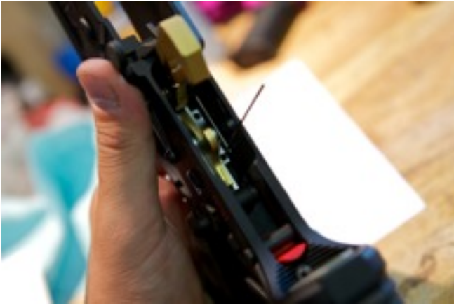
FIGURE 17 - ADJUSTMENT OF THE SET SCREWS
