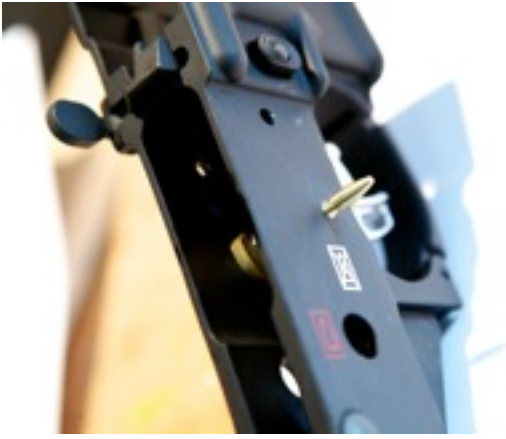
FIGURE 9 - TRIGGER PIN INSTALLED
