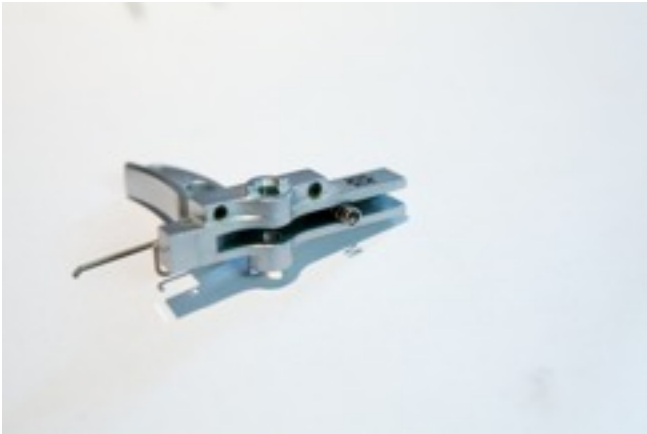
FIGURE 5 - DISCONNECTOR SPRING ON BATLTRIGGR
