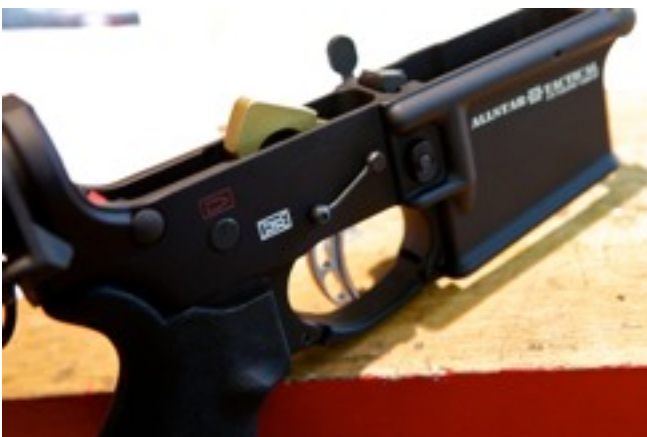
FIGURE 22 - TRIGGER INSTALL IS COMPLETE
